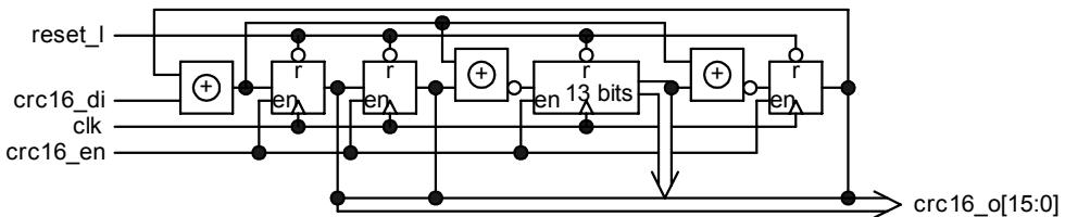
In general, CRC calculation is applied to a predetermined serial data field only. Accordingly, a certain timing signal to enable the CRC logic, "crc16\_en", must be made and provided.
