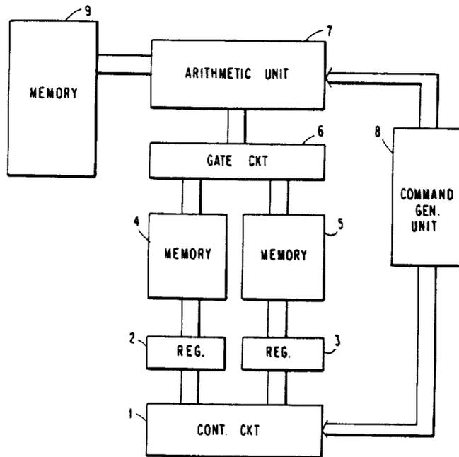
[54] **MULTIPLICATION CIRCUIT CAPABLE OF OPERATING AT A HIGH SPEED WITH A SMALL AMOUNT OF HARDWARE**
