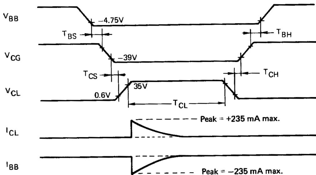
Note: The supply currents  $I_{BB}$  and  $I_{CL}$  diminish to almost zero within  $T_{CL}$
