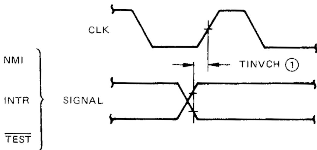
**NOTE:** ① Setup requirements for asynchronous signals only to guarantee recognition at next CLK.
