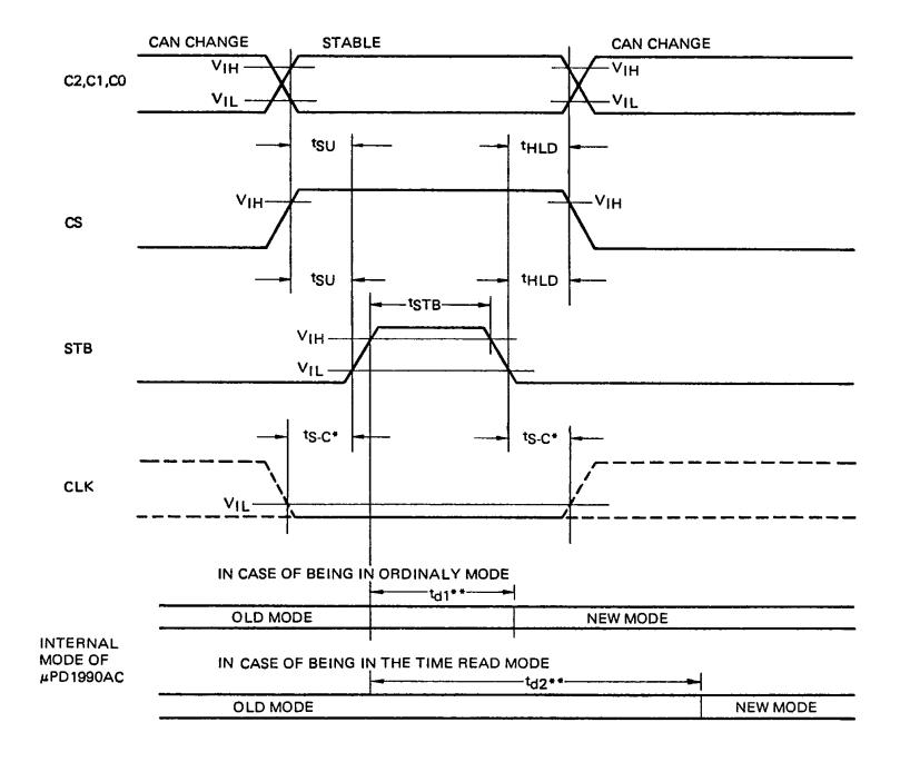
tsu = 2  $\mu$ s MIN. thld = 2  $\mu$ s MIN. tstb = 2  $\mu$ s MIN. td1 = 4  $\mu$ s MAX. (In case of being in ordinally mode.) td2 = 40  $\mu$ s MAX. (In case of being in the Time Read mode.) ts\_c = 2  $\mu$ s MIN.
