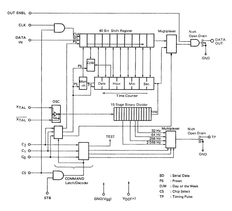
$f_{OSC} = 32.768 \text{ kHz}$  $V_{DD} = 2.0 \text{ to } 5.5 \text{ V}$
