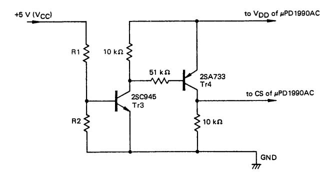
The Power Down of VCC line makes CS terminal inactive, with R1 and R2 resistors. The trigger level of this circuit is calculated as following.
