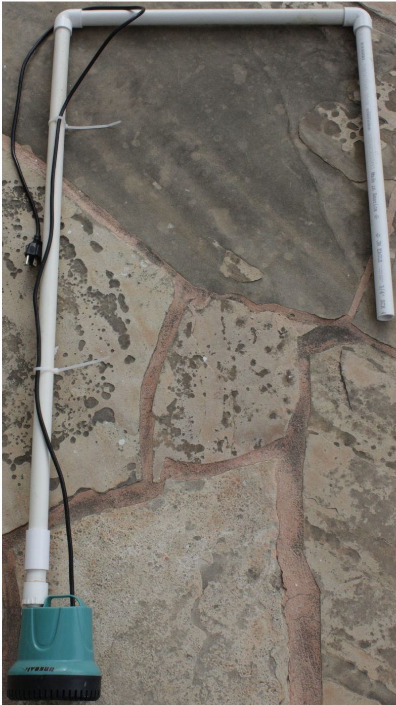
Pump & PVC pipe routing (A same pump, Common PVC pipes + Extension PVC pipes for 350 gallon water tank) For low profile 550 gallon water tank
