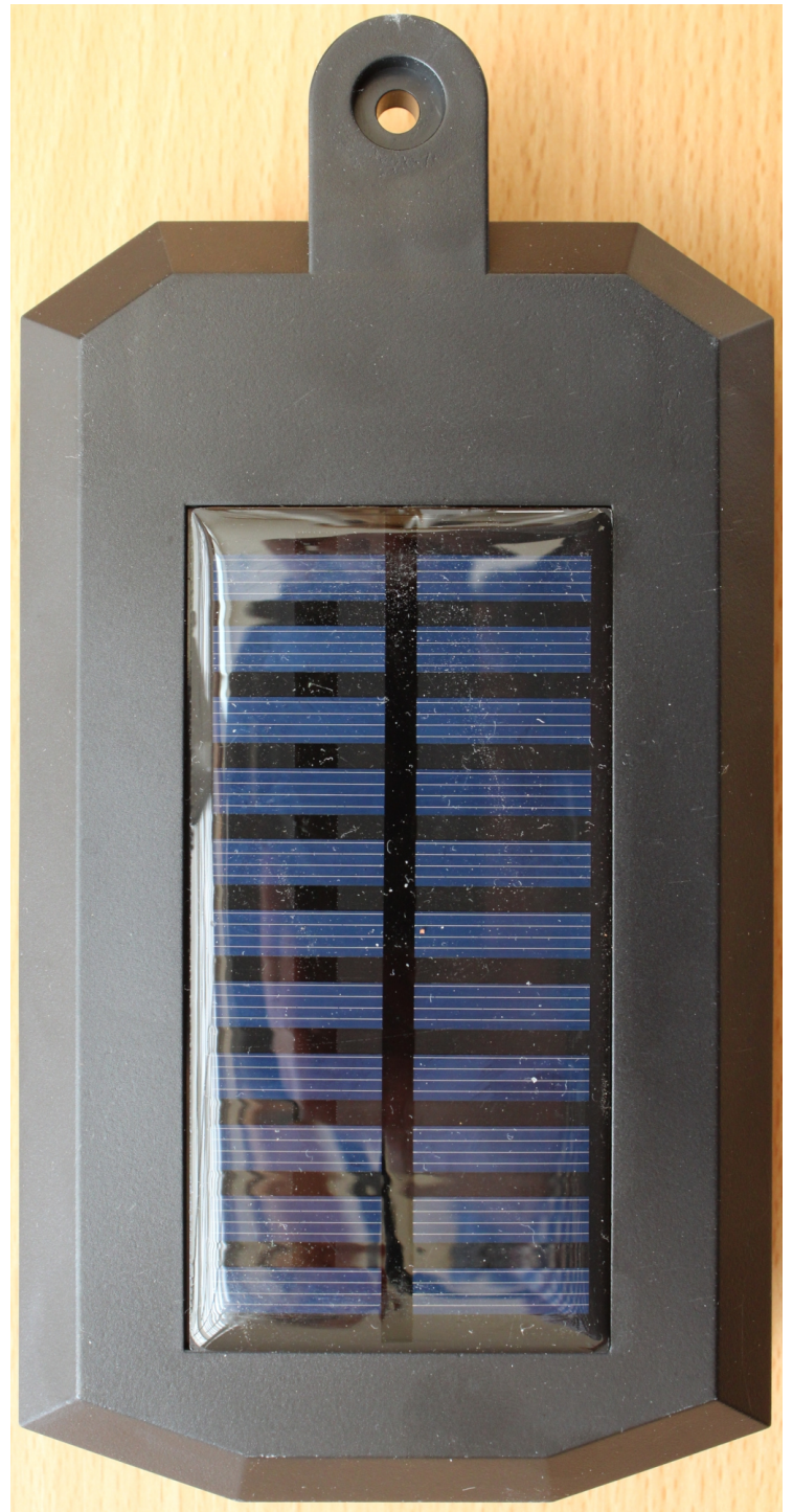
Solar Light #3 (52 (8 + 36 + 8) SMD (Surface Mounted Device) LEDs; no remote) under actual use
