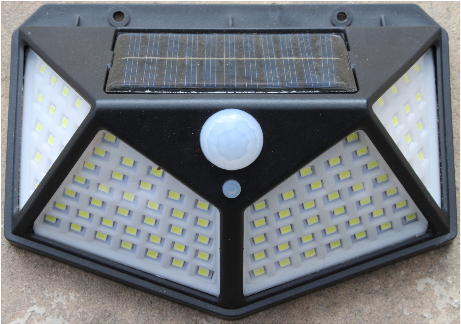
Solar Light #1 (100 (15 + 35 + 35 + 15) SMD (Surface Mounted Device) LEDs; no remote) under actual use
