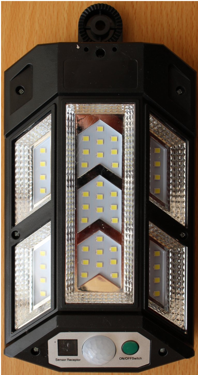
Solar Light #3 (52 (8 + 36 + 8) SMD (Surface Mounted Device) LEDs; no remote) under actual use
