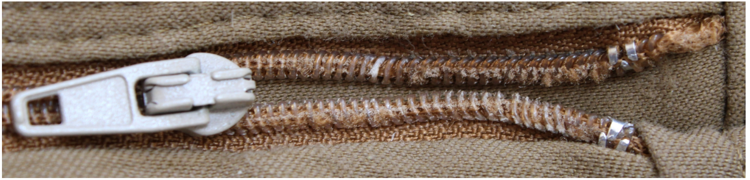
Lot of yarn waste near top stops (Probable cause of zipper slide derailment)
