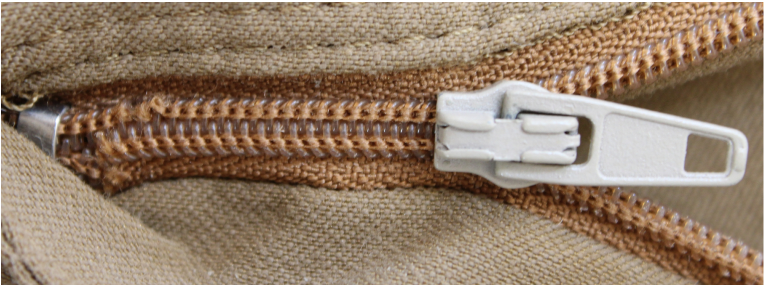
Success (Lower 4 teeth engaged manually by using finger nails and a small minus head driver)
