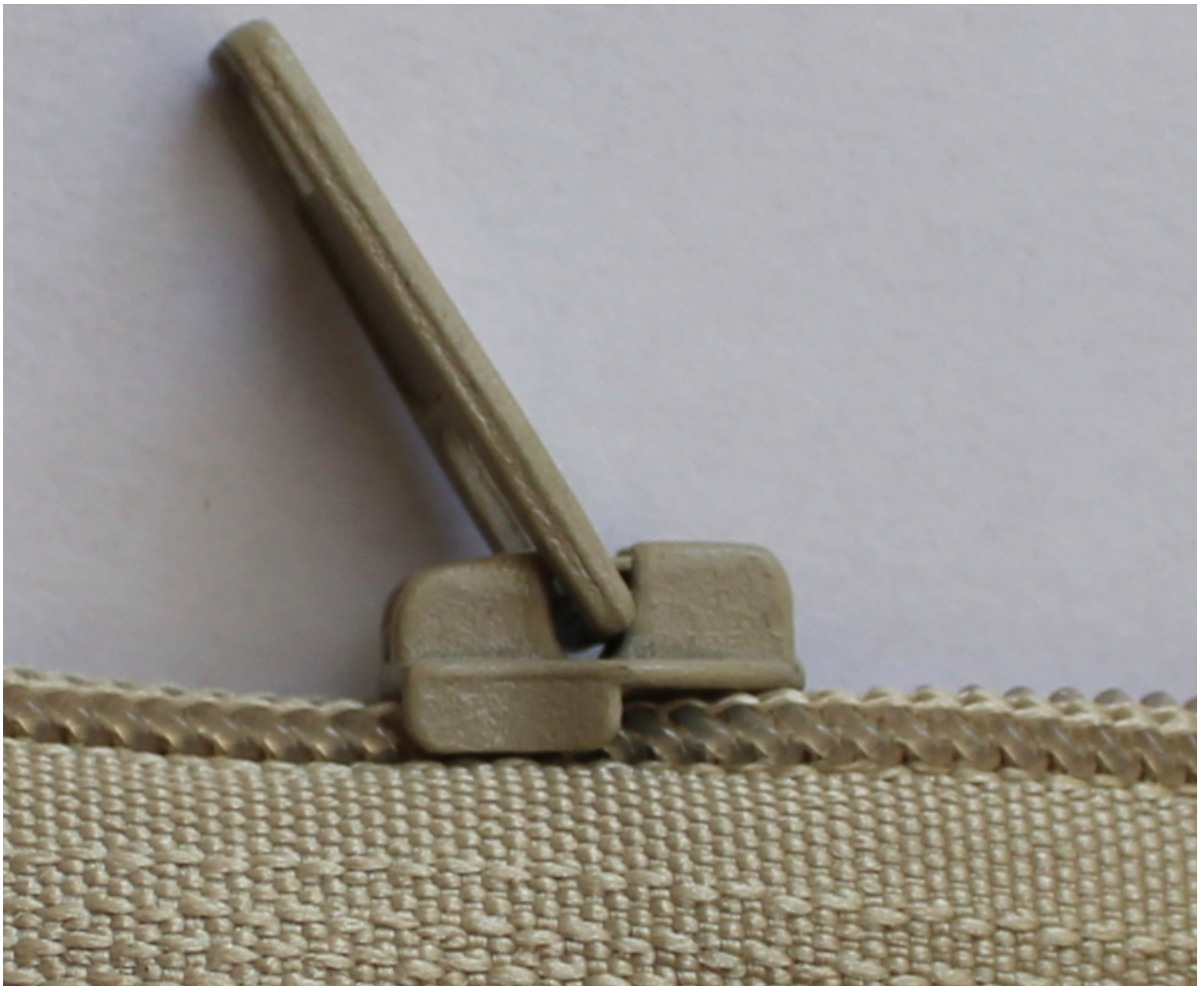
Side view of slider (3mm height nylon coil, side walls of slider engage teeth interchangeably)
