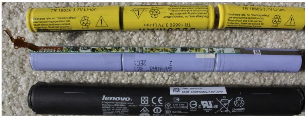
Inside of battery pack (three 3.75V Li-ion batteries in parallel)
