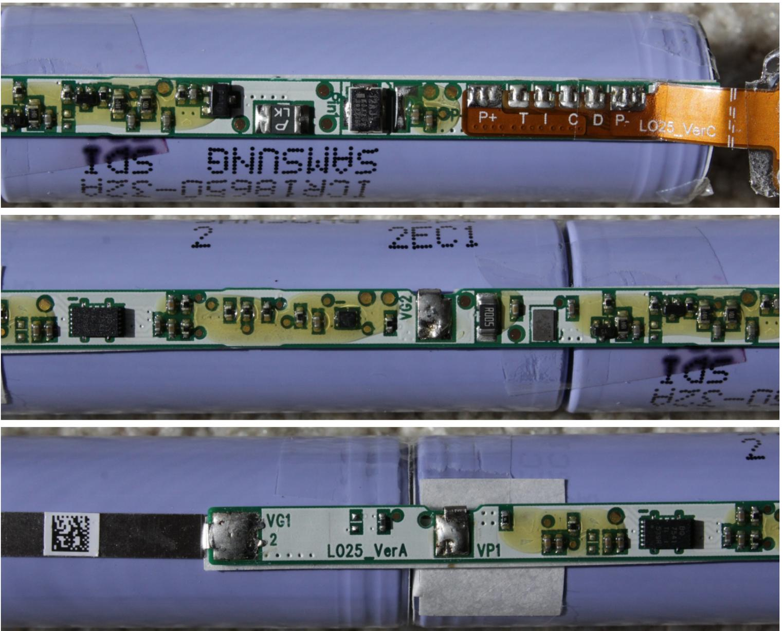
Details (with battery controller board)
