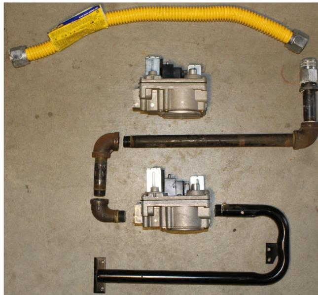
After Removing Gas Valve Disconnecting Gas Pipes (Old Gas Valve (Up), New Gas Valve (Down))
