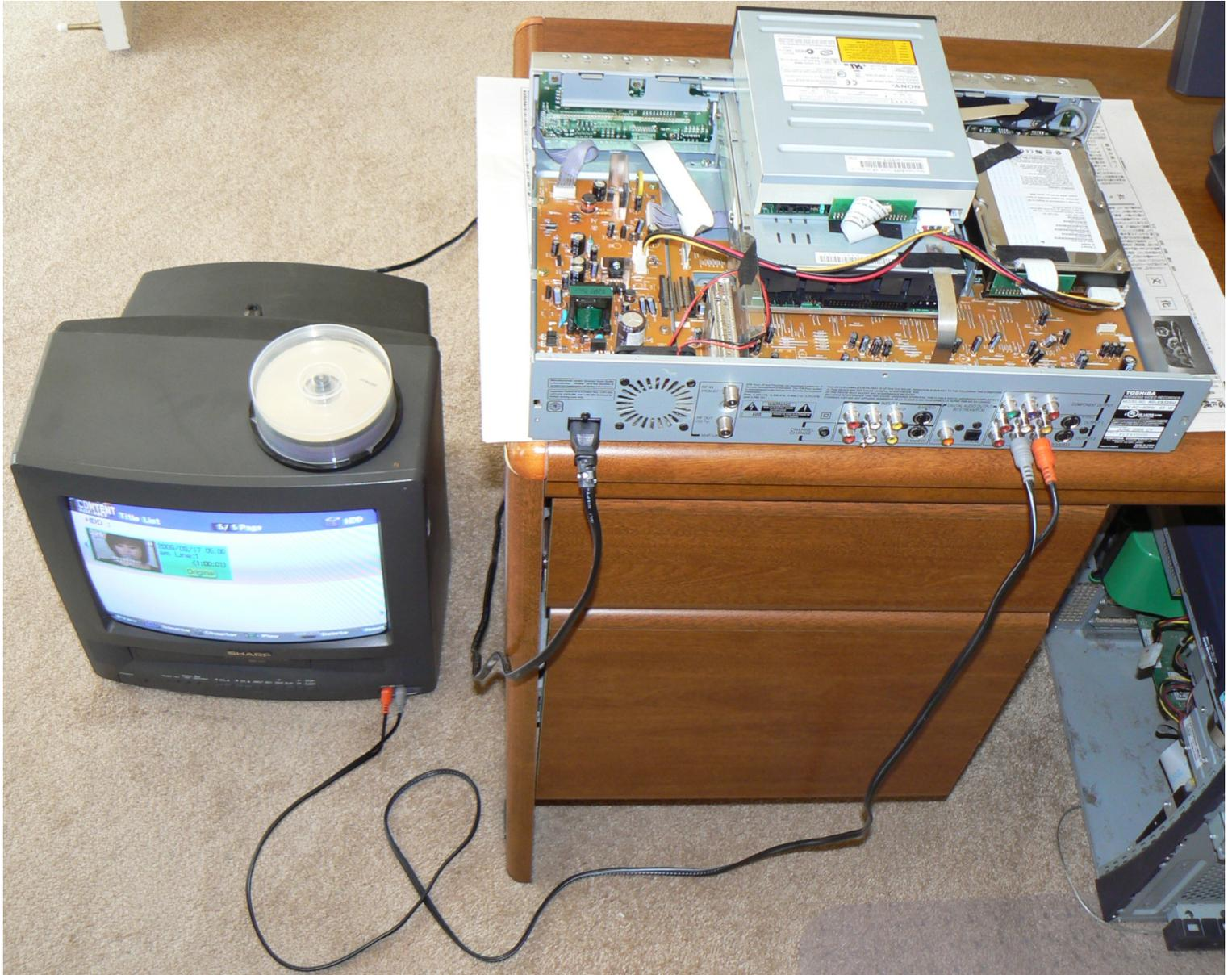
DVD-RW Drive with ATA Parallel Interface Piggy-backed, Analog TV Connected by Composite Video and Audio
