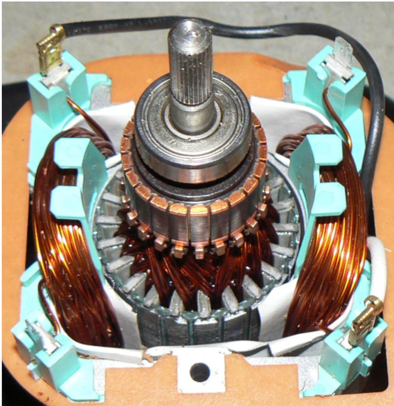
Rotor with Windings & Commutator, Stator Windings, Ports
