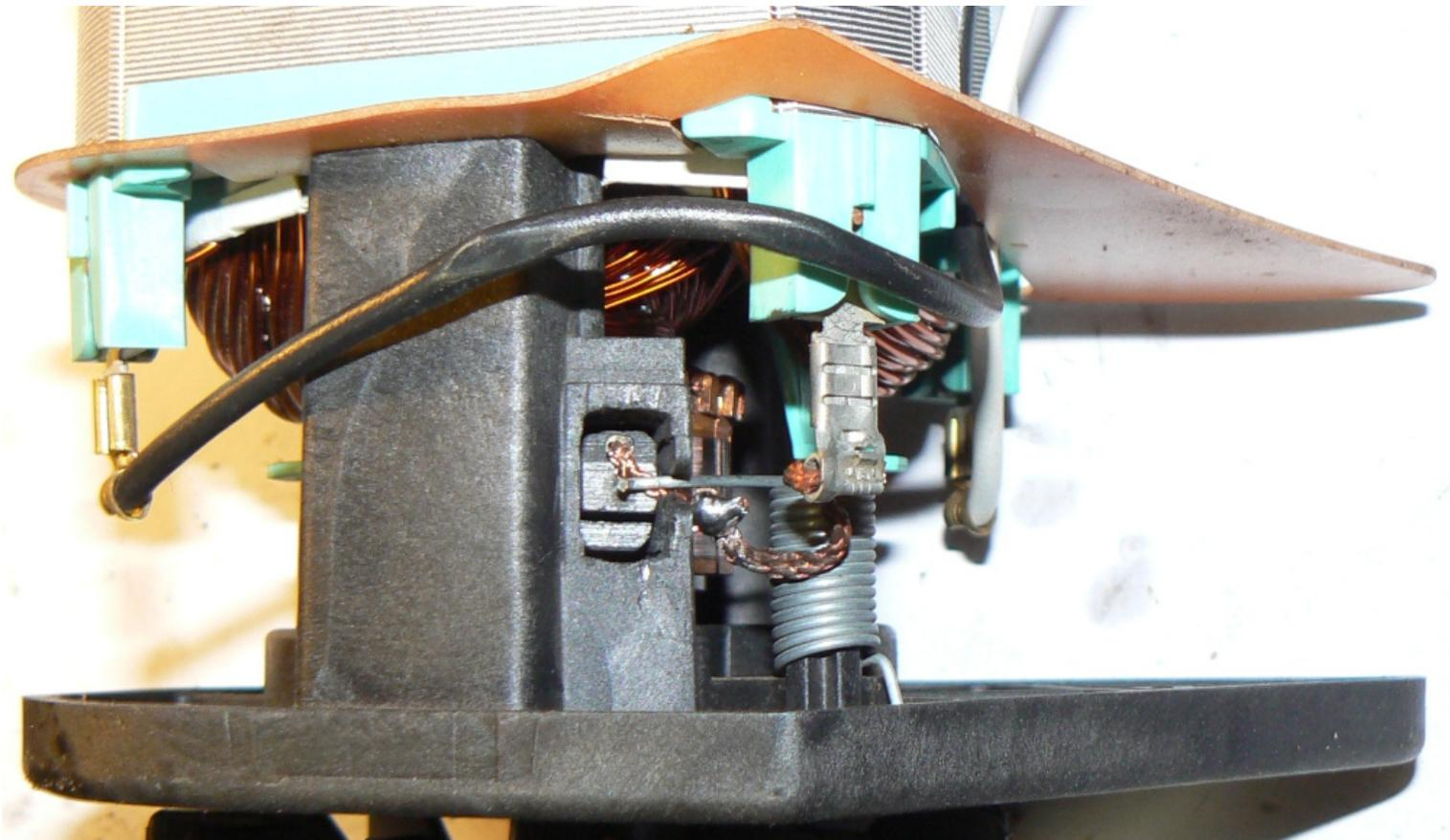
Replaced Carbon Brushes & Connected to the Terminal
