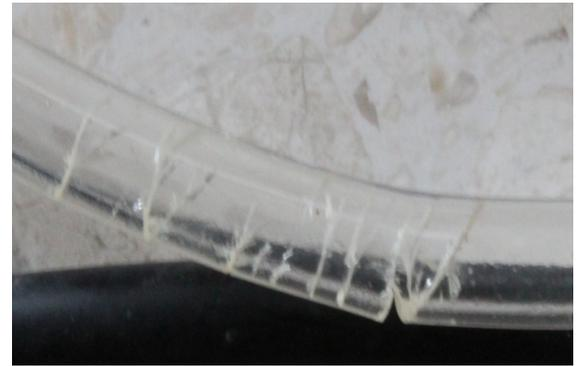
Water Leaked Due to Seriously Cracked Hose (Low Quality Hose Used)
