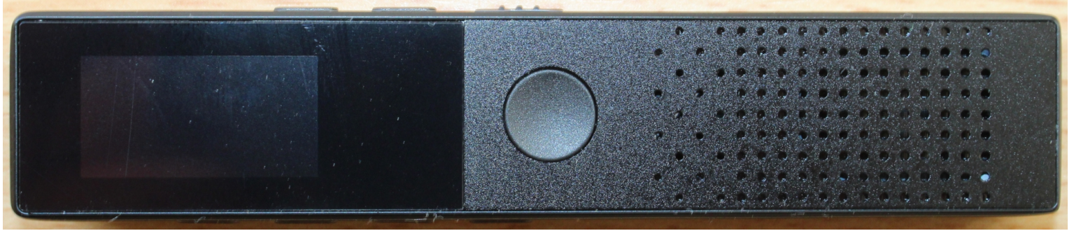
Body size; 10 cm (H) x 2 cm (W), Display size; 22.5 mm (H) x 11.5mm (W), "Record/Save", Speaker
