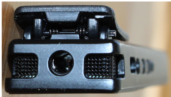
3.5 mm headphone plug, Right & left stereo microphone, Clip (Up)
