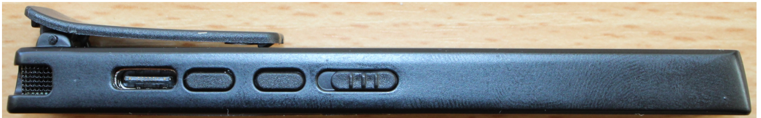
Microphone (R), USB-C port (Charge battery and access 64GB flash memory), "VOL+", "VOL-", "ON/OFF"
