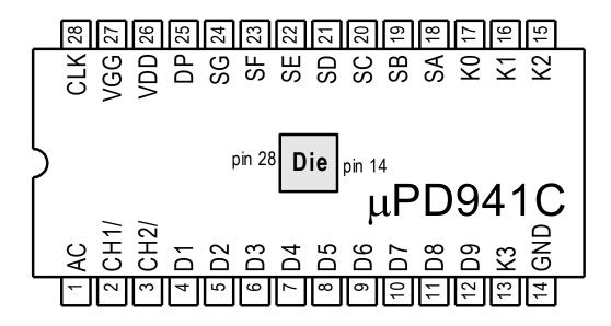
Pin association of next page die photo exactly reflects the die position mounted on the island of the base ribbon.
