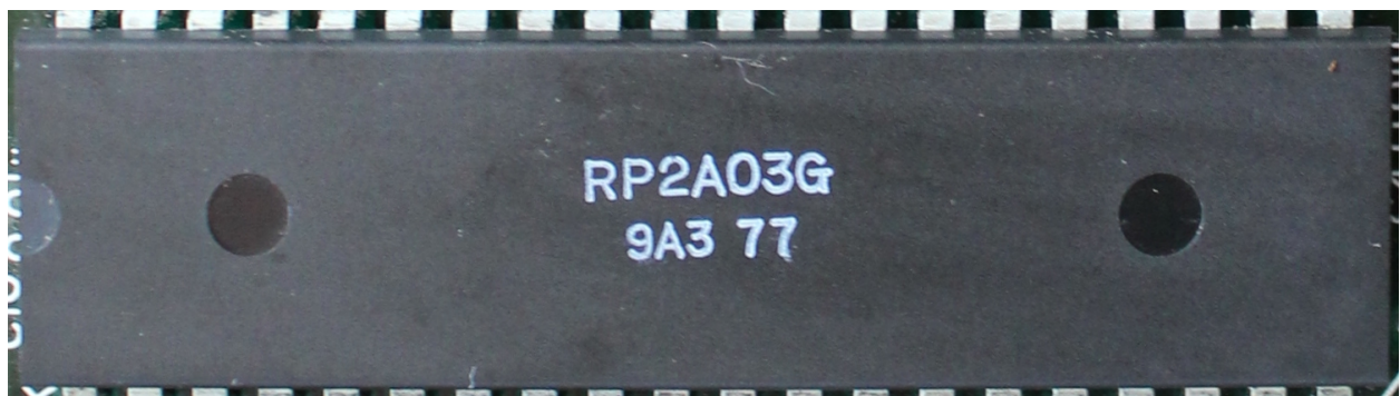
Ricoh RP2A03 (8 bit CPU for Nintendo Family Computer HVC-001, 40 pin)
