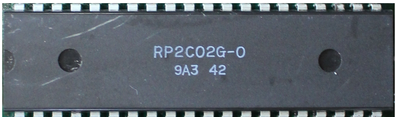
Ricoh RP2C02 (Picture Processing Unit for Nintendo Family Computer HVC-001, 40 pin)
