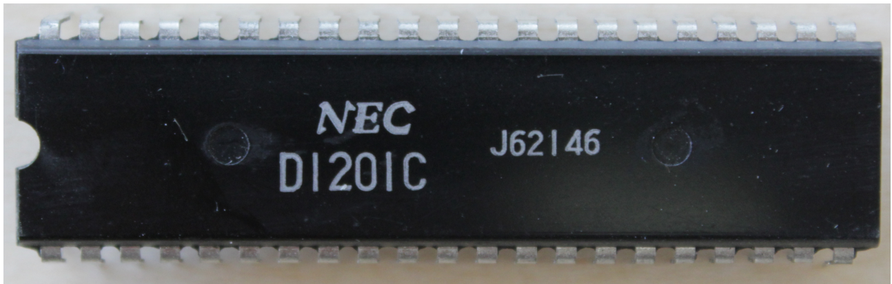
NEC \mu PD1201C (12 Digits Desk-top Calculator LSI with Printer Control I designed, 42 pins)
