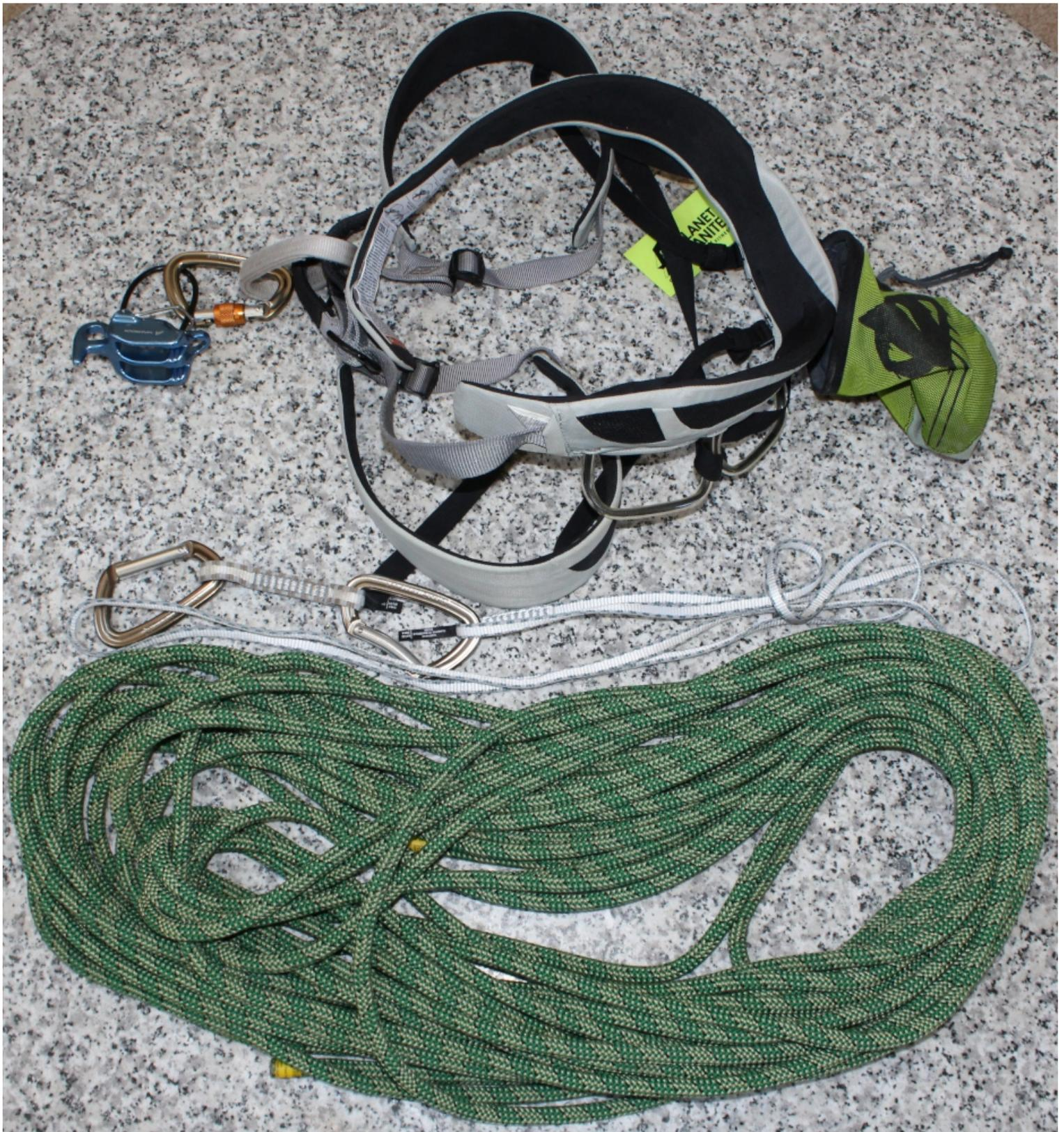
Complete Set of Roof Work Gear without Nonskid Shoes
