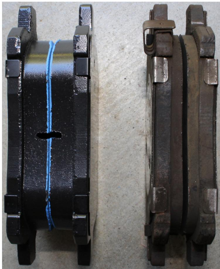
Thick New & Thin Old Brake Pads
