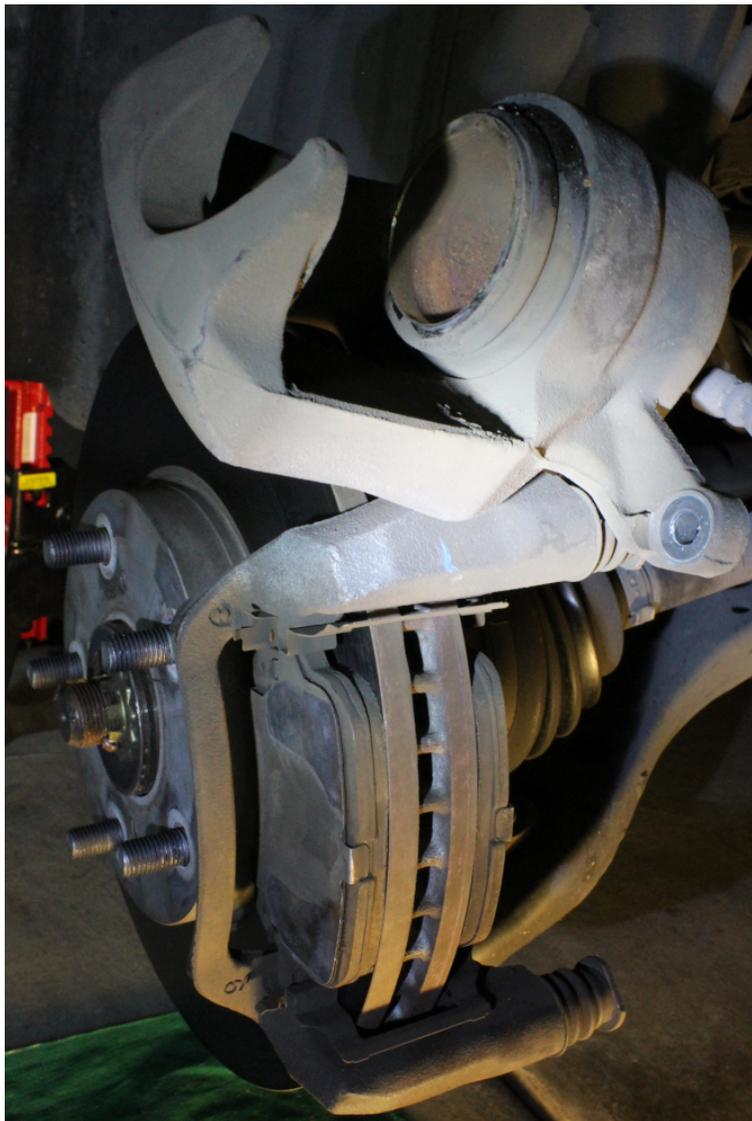
Brake Pads Exposed (Up; Brake Caliper Detached)
