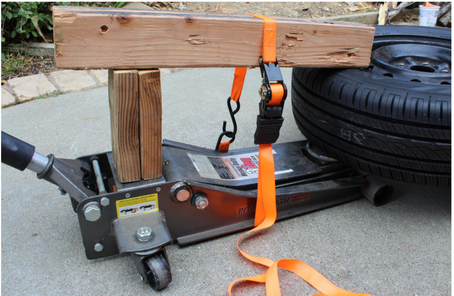
Efficient Low Cost Beads Release System
