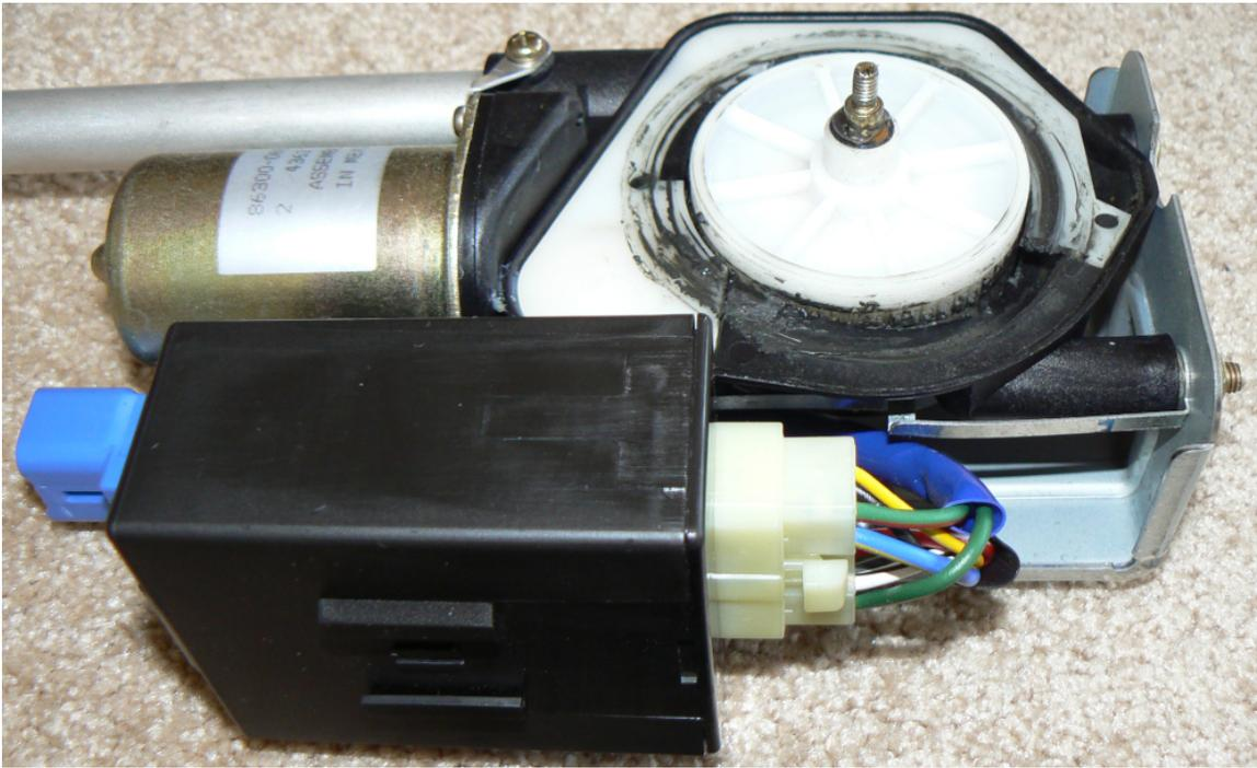
Powered Antenna Motor & Gear Unit
