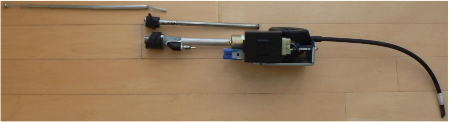
Broken Antenna (Antenna drive cable broke & shortened)
