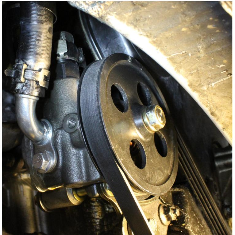
Replaced (Clean; No Oil Leak)
