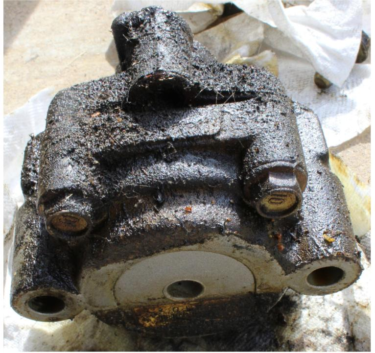
Old Power Steering Pump Fully Being Drenched by Power Steering Oil
