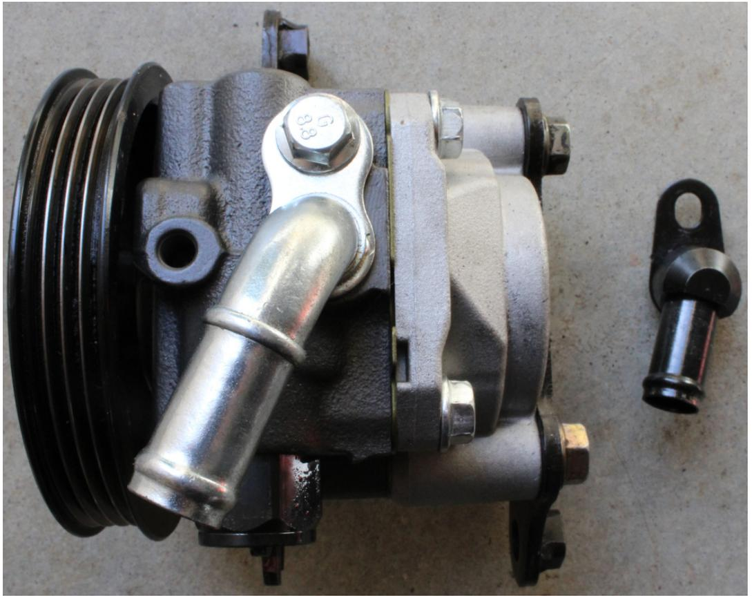
Return Hose, Bracket, New Power Steering Pump Assembled with Parts
