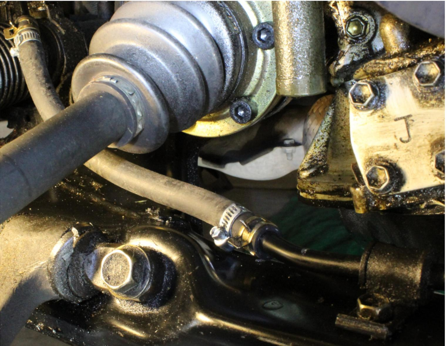
Power Steering Pump Pressure Feed Tube Replaced
