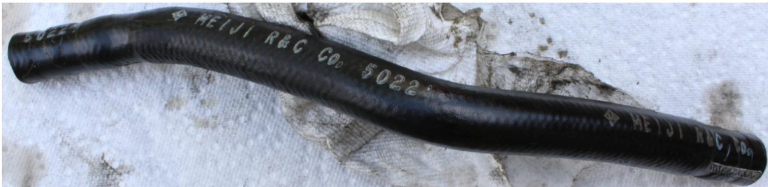
Old Power Steering Pump Pressure Feed Tube with Crack
