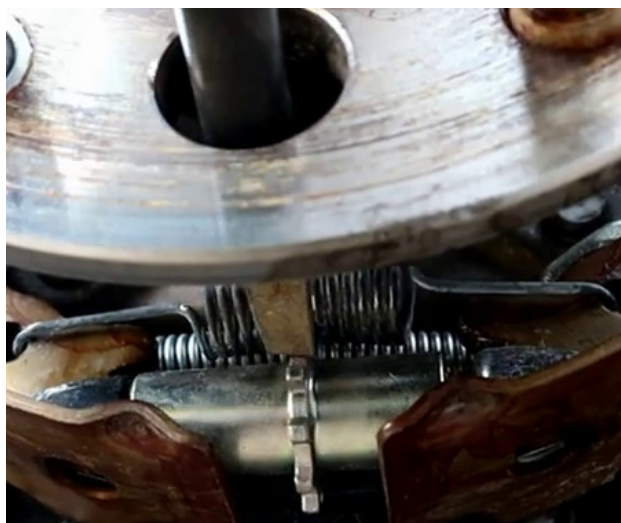
Rotate adjuster teeth up to loosen, down to tighten
