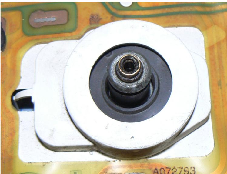
Cable Receptacle on New Instrument Cluster
