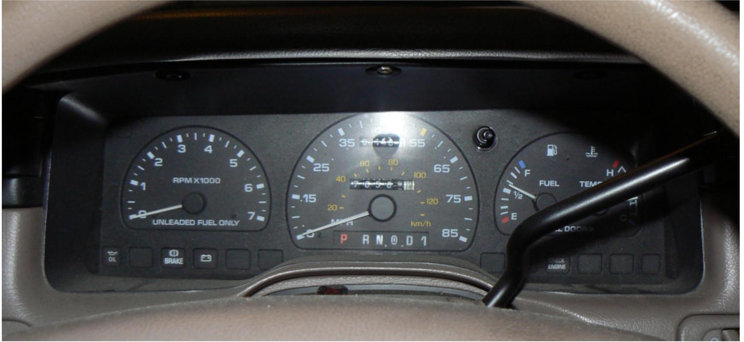
Old Speedometer (Center of Instrument Cluster) Installed
