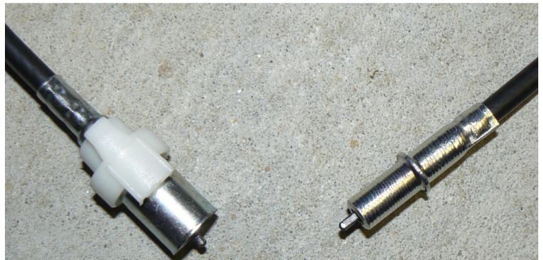
New Cable (Left to speedometer, Right to cable linkup)
