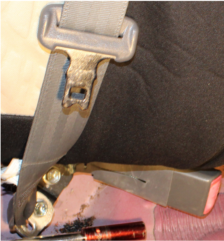
No locking hole in chassis (Design flaw) for middle rear safety belt bridge anchor makes arbitrary rotation
