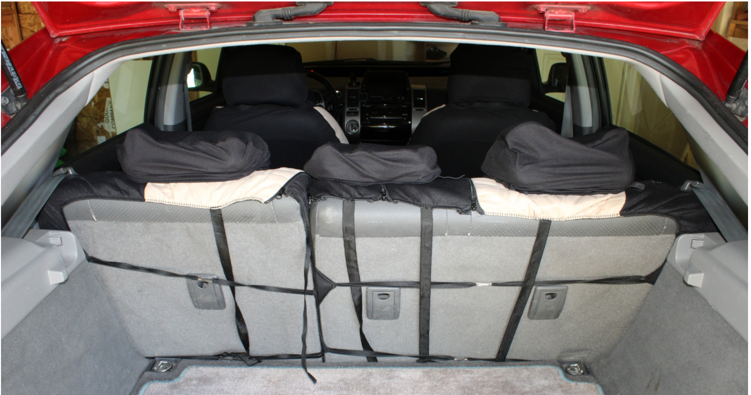
Cross straps with adjustable buckles (Vertical) and elastic loops using metal clips (Horizontal)
