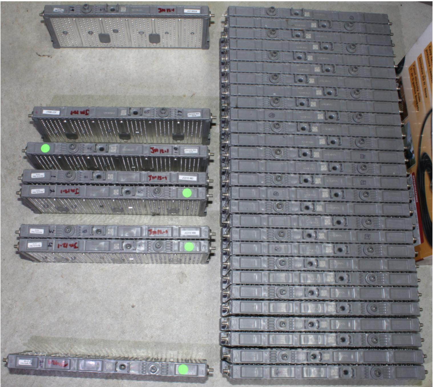
8 Battery Modules for Replacement (Left; N7, N5, N6, N1, N2, N3, N4, N8) vs. Target (Right; #1 - #28)
