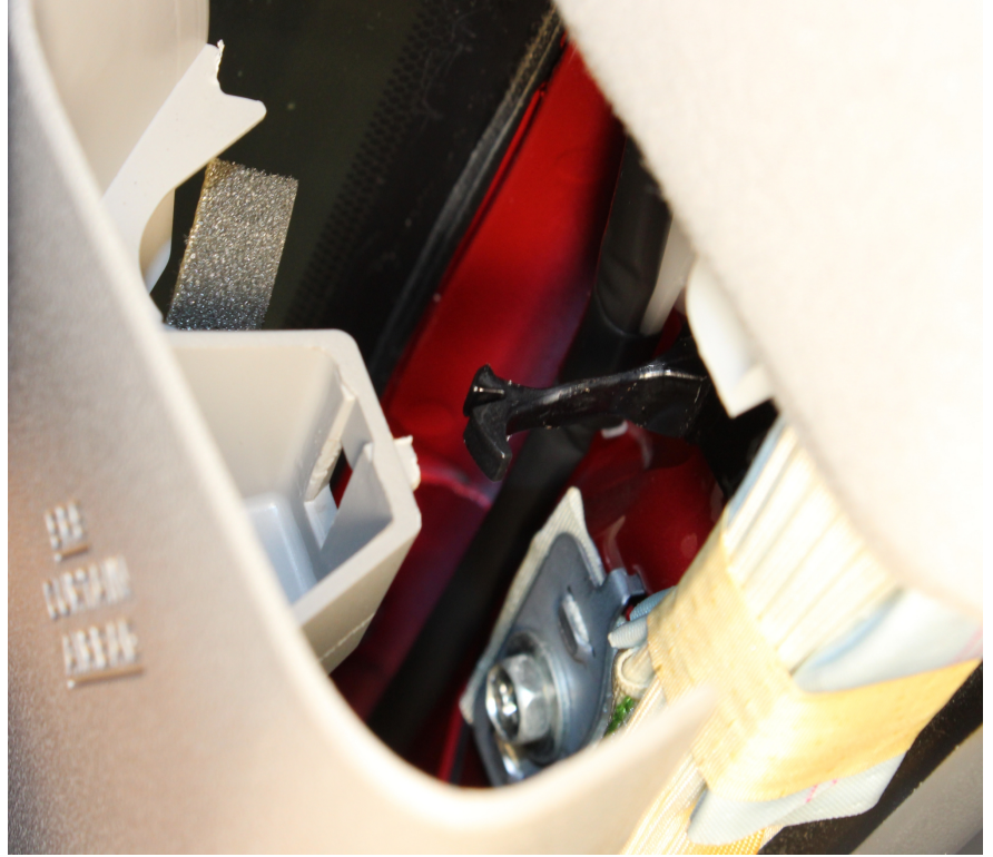
Elastic Clips to be rotated 90 degrees to release
