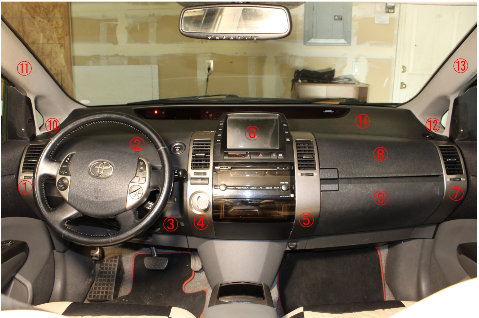
Instrument Panel disassembly sequence (from ① to ⑭)
