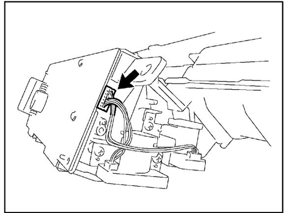
10. Install Meter Circuit Plate No. 4.
