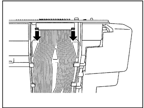
7. Remove Meter Circuit Plate No. 4.
