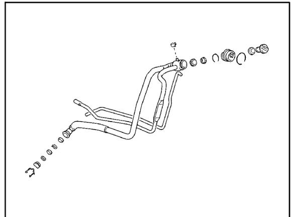
8. Install Fuel Tank Filler Pipe Sub-assembly.
