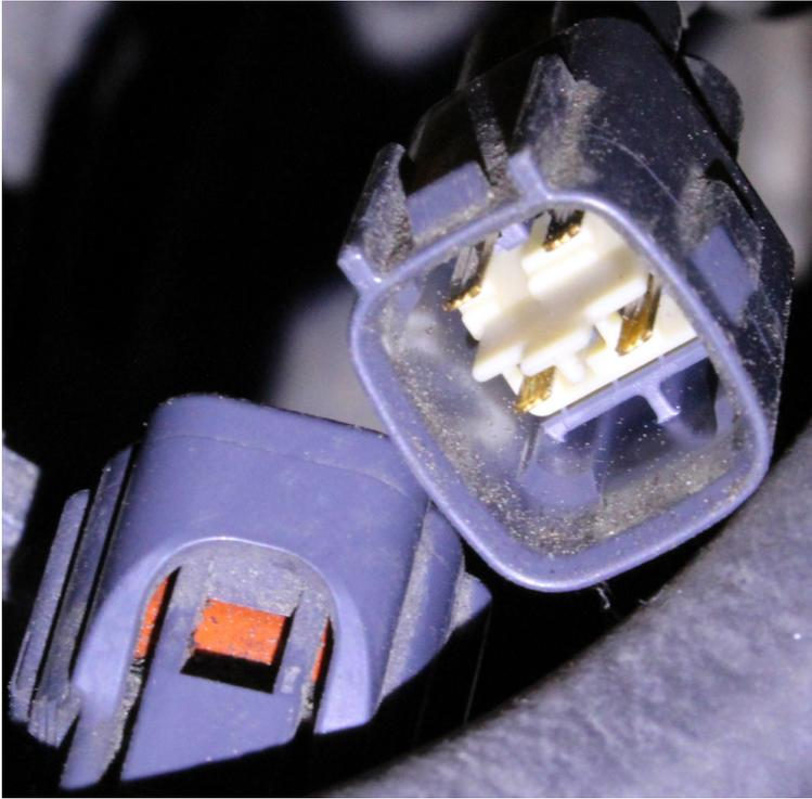
Oxygen Sensor Connector Disconnected (System Side)
