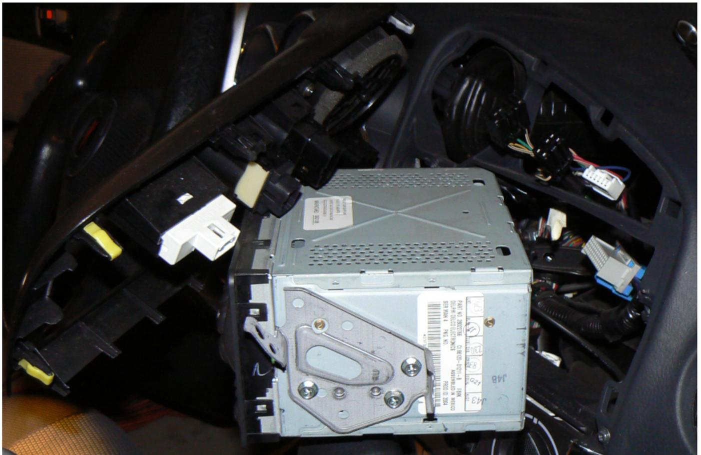
Old Car Stereo Removing from Console
