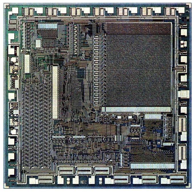
Higher resolution Die micrograph of  $\mu PD941C$  (Derivative of  $\mu PD940C$ ) based upon this mask layout design
