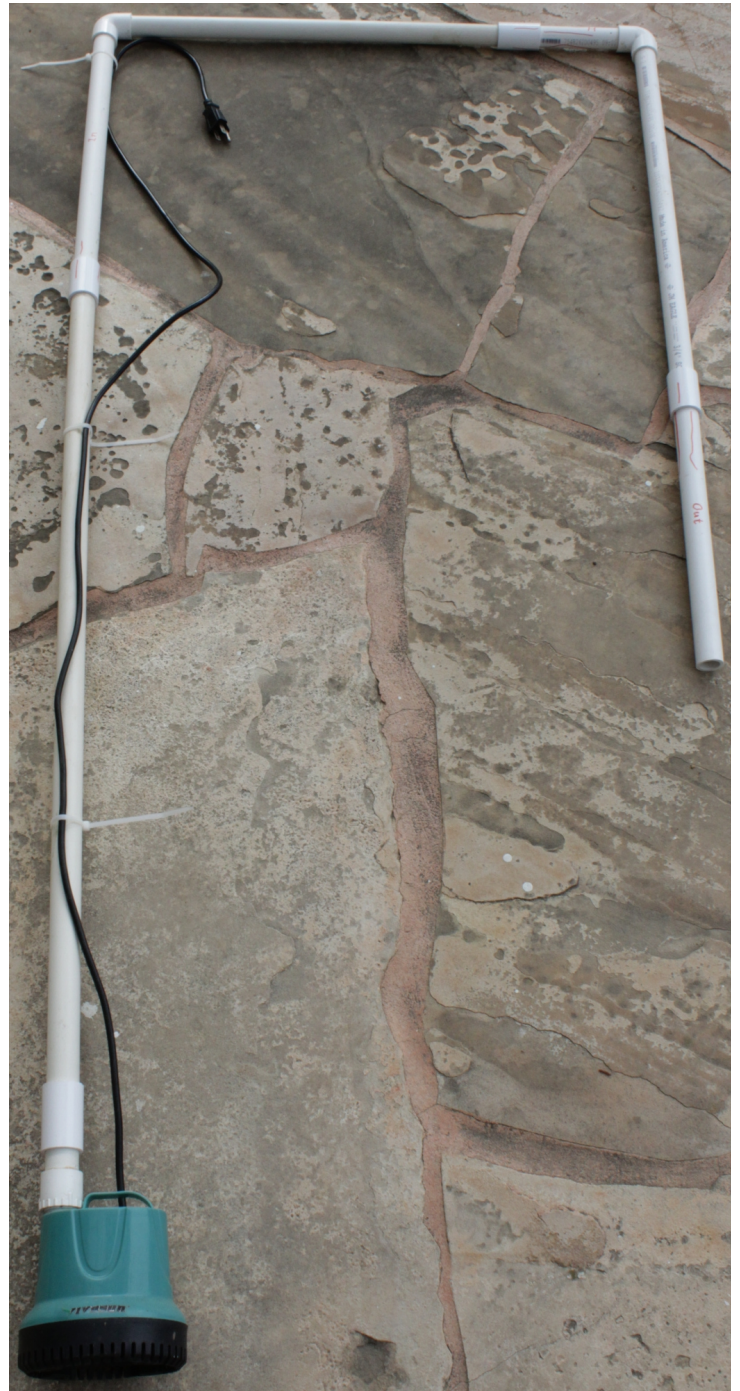
Pump & PVC pipe routing (A same pump, Common PVC pipes + Extension PVC pipes for 300 gallon water tank) For low profile 550 gallon water tank
