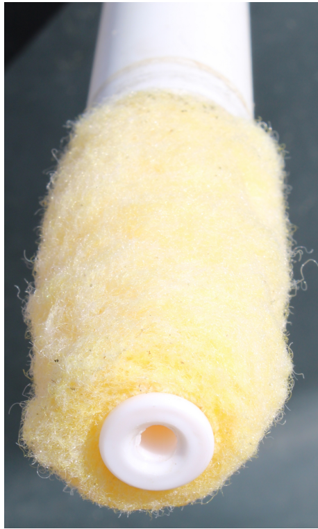
wet paint roller passing in pipe
