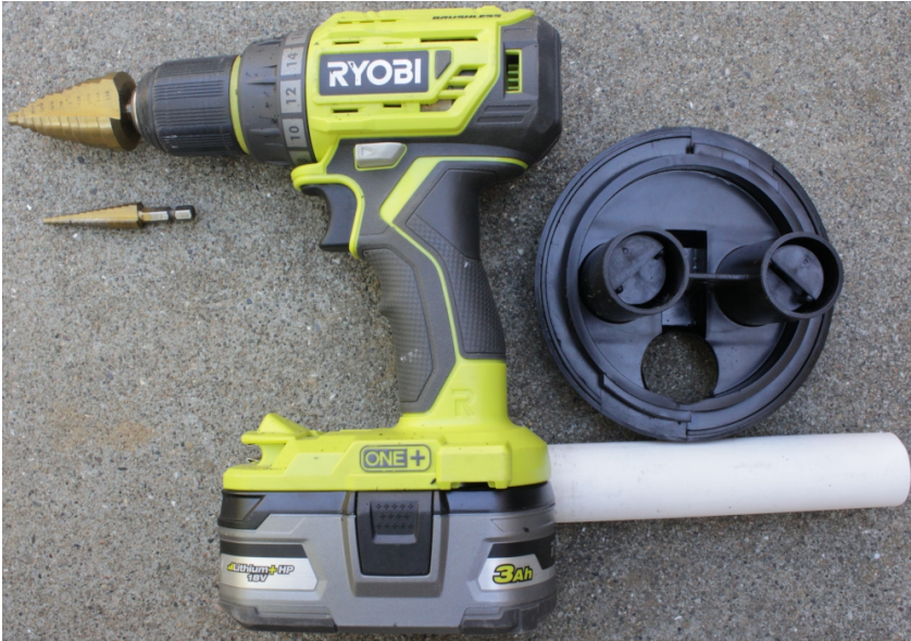
Making a hole on water inlet lid by two reamers & Drill)
