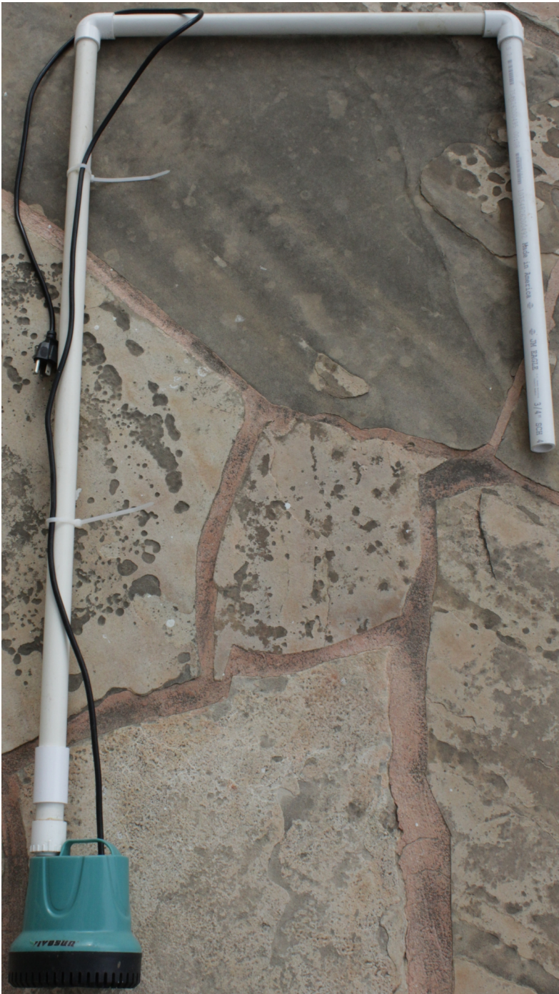
Pump & PVC pipe routing (A same pump, Common PVC pipes + Extension PVC pipes for 300 gallon water tank) For low profile 550 gallon water tank
