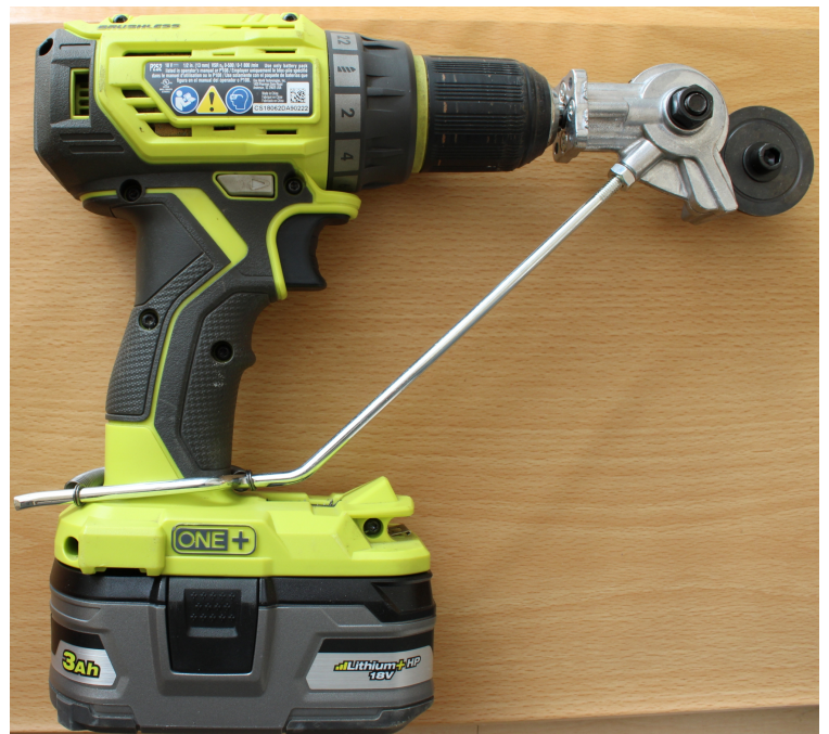
How to assemble sheet metal cutter to cordless drill
