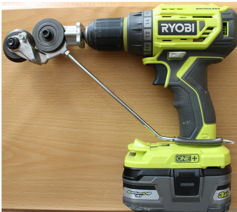
How to assemble sheet metal cutter to cordless drill
