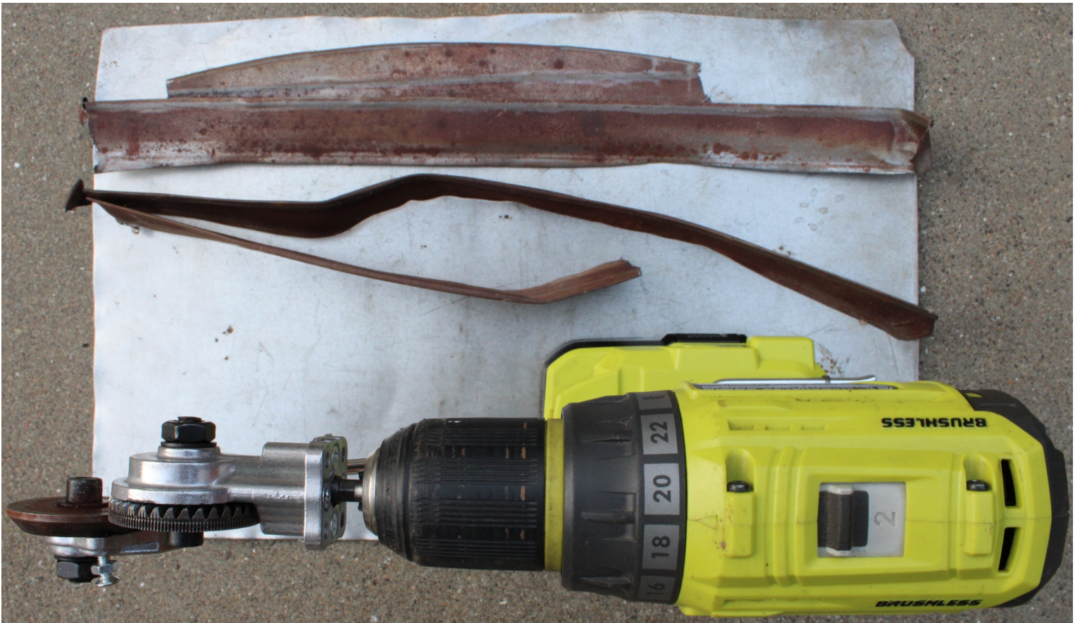
Successfully made a sheet metal by using a sheet metal cutter
