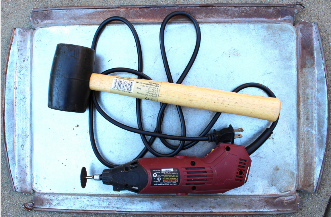
Cut four sides by rotary tool and flatten by rubber mallet
