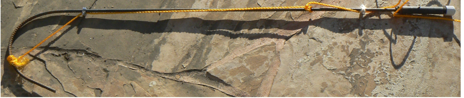
Hand-made Branch Puller (Hook Rounded Rebar to Branch, then, Pull Rope down)
