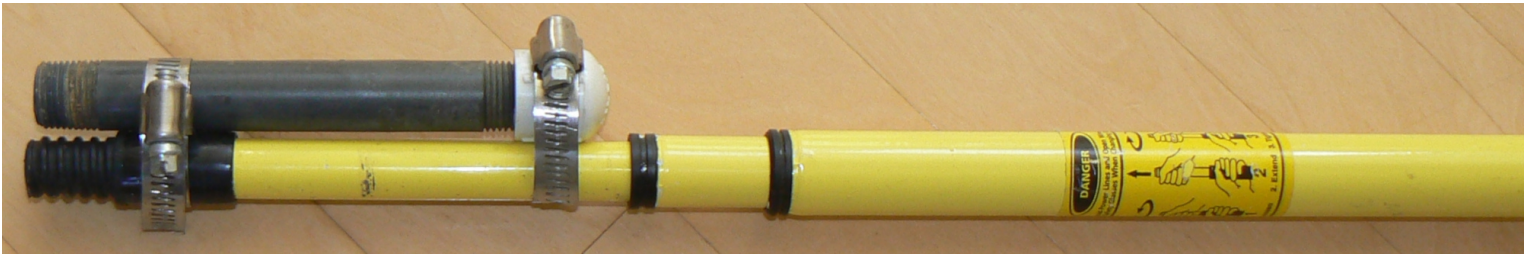
Rebar Pipe Socket at Front Edge of Extendable Rods
