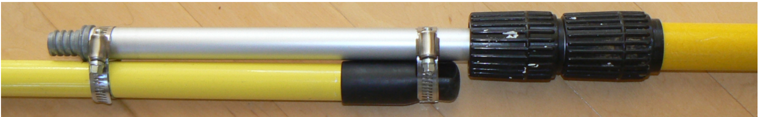
Connection between Two Extendable Rods using Hose Clamps
