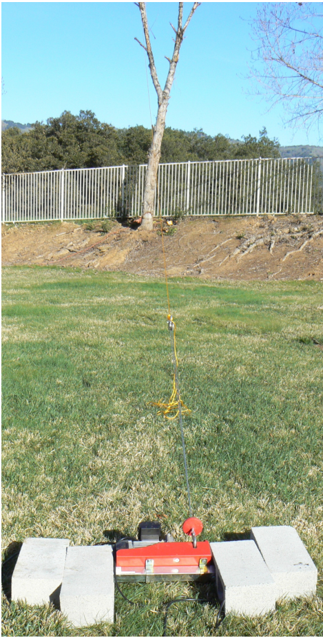
Pulling Rope by Winch
