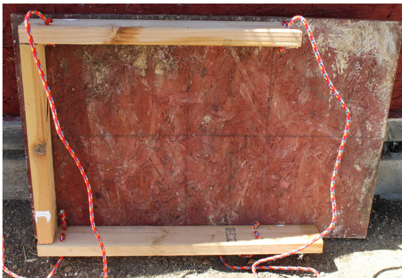
Hand-made Slope Boat to Carry Skirts & Stems Sliding from Top of the Slope down to Bottom by Two People
