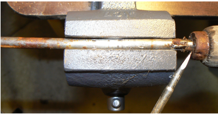
Removing Metal Weed Sticker Portion Fixing by Vise
