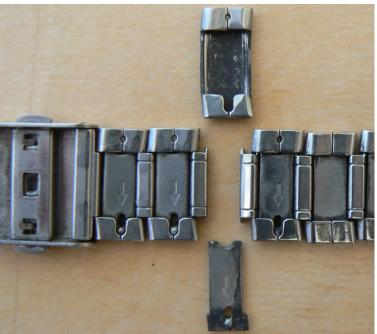
Removing Metal Section Block
