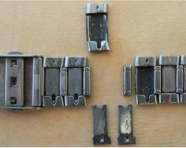
Removing Metal Section Block
