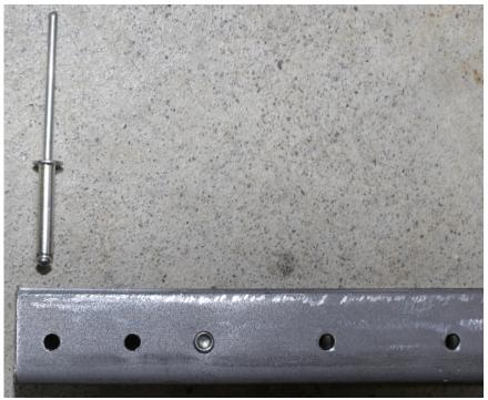
$1/8" \times 5/8"$  Rivet for Top Guide of New Channel Balance
