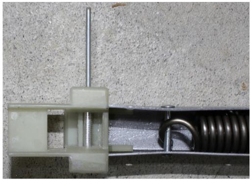
$1/8" \times 5/8"$  Rivet Passed through Hole to be Fixed
