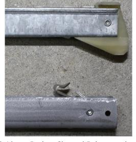
Top Guide on Broken Channel Balance to be Removed Bottom Guide on Broken Channel Balance to be Removed
