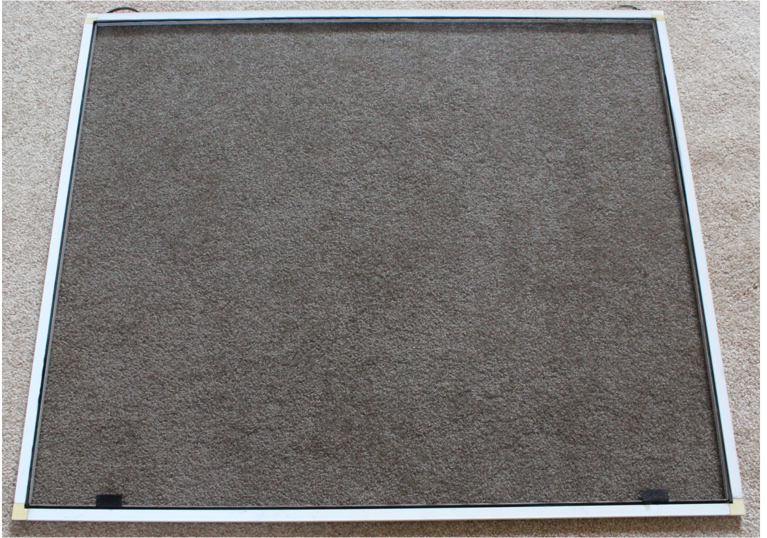
Done (Screen Tension Looks Good, Extra Spline Needs to be Cut)
