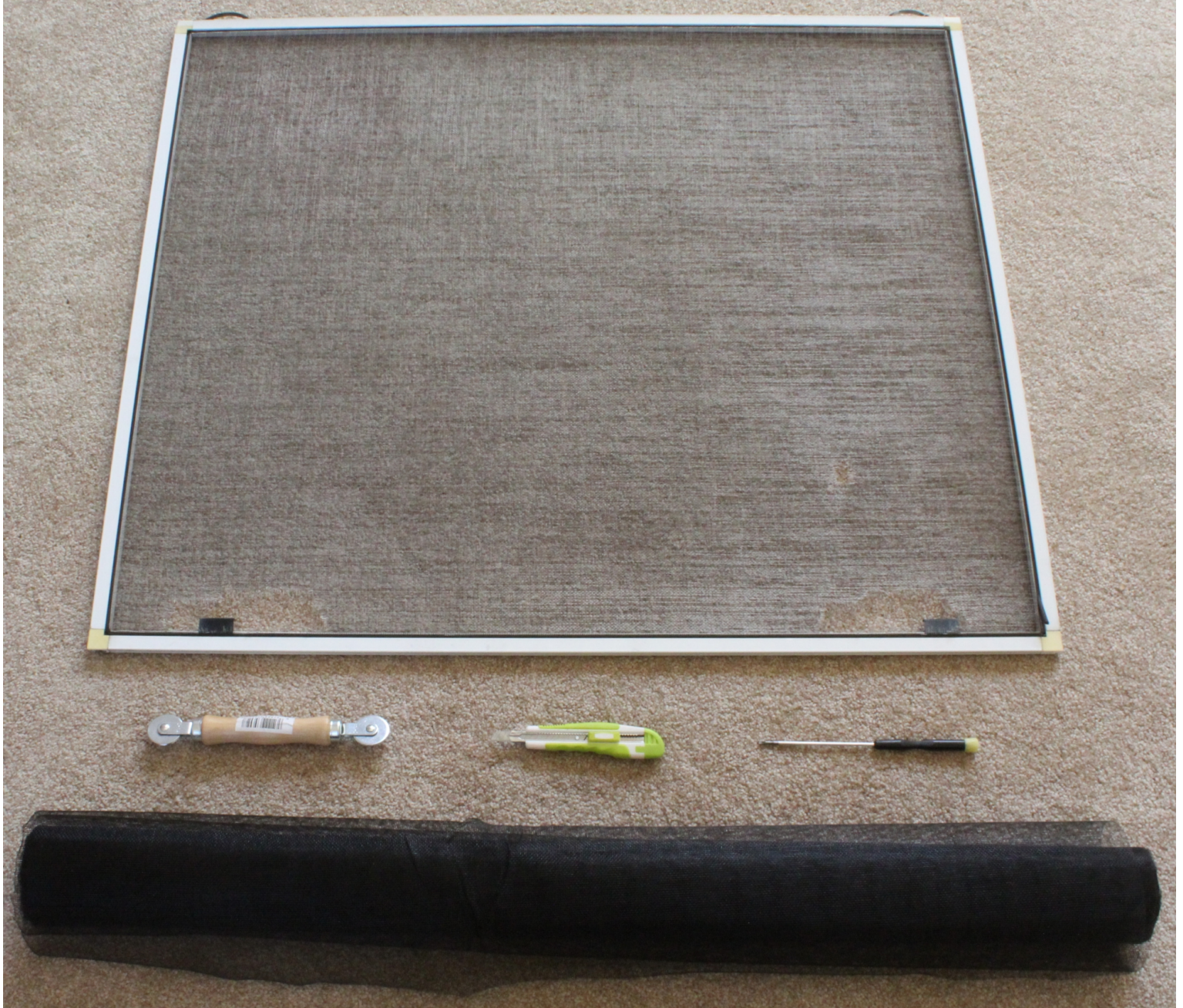
Window Screen to be Replaced, Spline Roller, Knife, Driver, Roll of New Screen (Old Spline still under Use)
