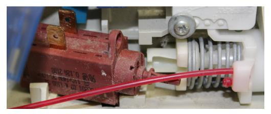
Removing Malfunctioned Wax Motor (Brown Shaft)
