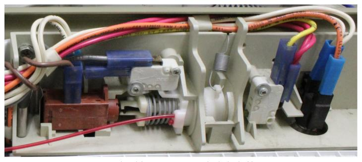
Replaced (New Wax Motor with Black Shaft)
