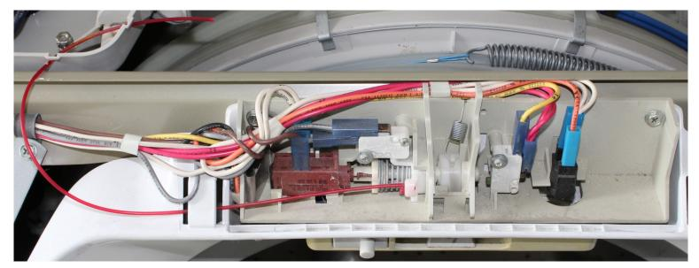
Malfunctioned Wax Motor (Brown Shaft), Micro Switches, etc.
