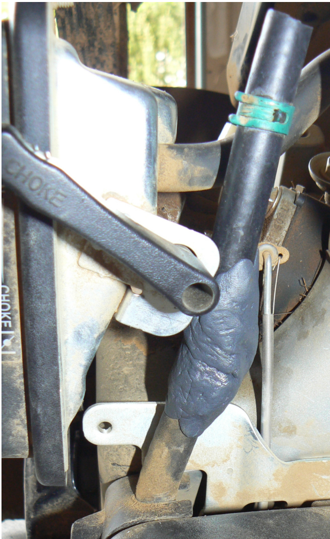
Connected between Old & New Hose by Epoxy Putty
