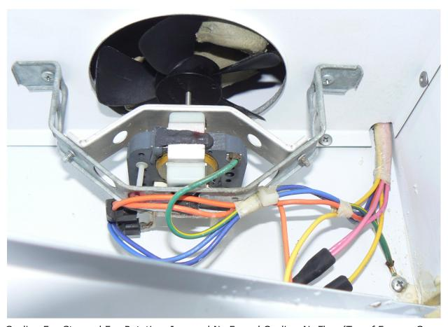
Putty on Cooling Fan Stopped Fan Rotation, Incurred No Forced Cooling Air Flow (Top of Freezer Compartment)
