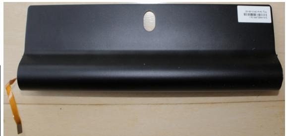
® Registered Trademark of Lenovo Model Name (型號/型号): L14C3K31 执行标准:GB/T 18287-2013 NOM 3.75V == 36.0Wh ,9600mAh MIN 3.75V == 34.8Wh ,9300mAh Rechargeable Li-ion Battery 1ICR19/65-3 二次鋰電池組 Manufactured for Lenovo Cell made in Korea Pack processed in China
