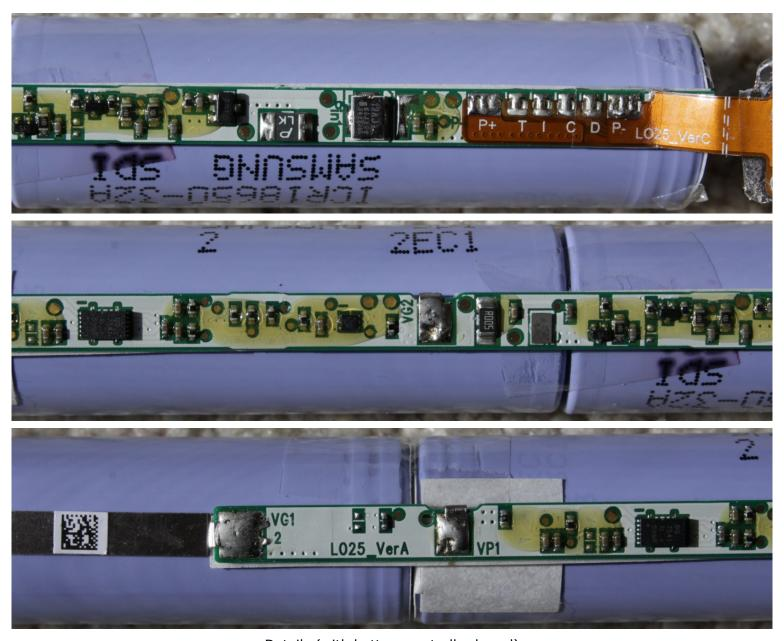
Details (with battery controller board)
