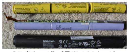
Inside of battery pack (three 3.75V Li-ion batteries in parallel)
