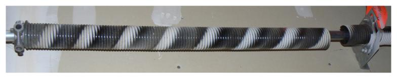
Torsion Spring (Left) of Garage Door Broke
