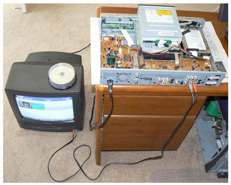
DVD-RW Drive with ATA Parallel Interface Piggy-backed, Analog TV Connected by Composite Video and Audio
