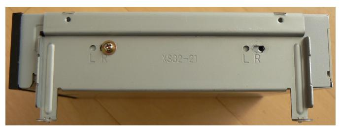
Bolt Hole Position of Side Bracket had to be Shifted Backward a bit
