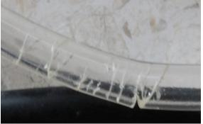
Water Leaked Due to Seriously Cracked Hose (Low Quality Hose Used)
