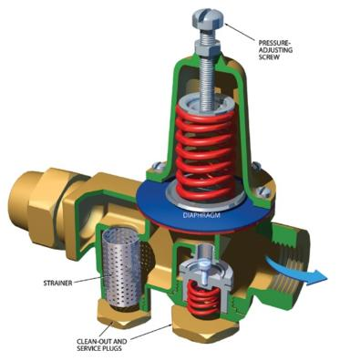
Water Pressure can be Adjusted by Adjusting Screw
