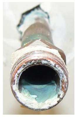
Sediments in 1/2" Copper Pipe Inlet
