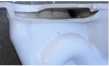
Flush Water Inlet (Cross Section View)
