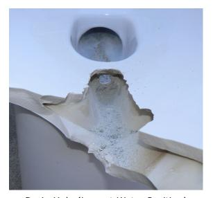
Drain Hole (Lowest Water Position)
