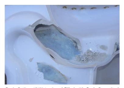
Drain Path until Water Level Filled with Scale Deposited
