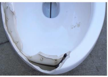
Flush Water Flows Rear Surface of Bowl and Drain
