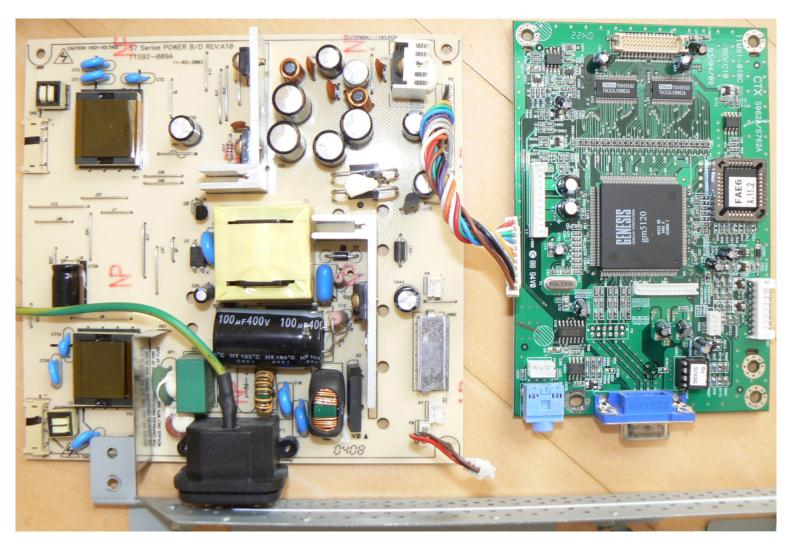
Power Supply & Controller with VGA video connector & Audio Connector
