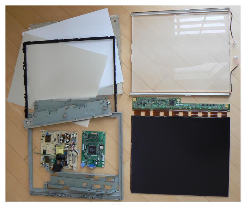
Whole Aspect Monitor Frame, Two Back Lights with Diffusion Sheet, Power Supply, Controller, Driver, LCD Flat Panel
