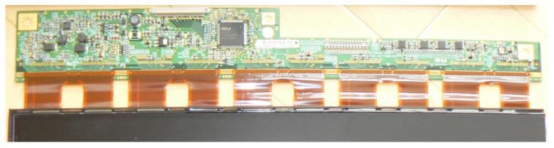
Row & Column Drivers and LCD Flat Panel Connected by FFC (Flexible Flat Cable)
