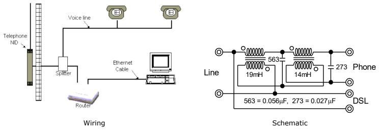
DSL Splitter with DSL Pass Through
