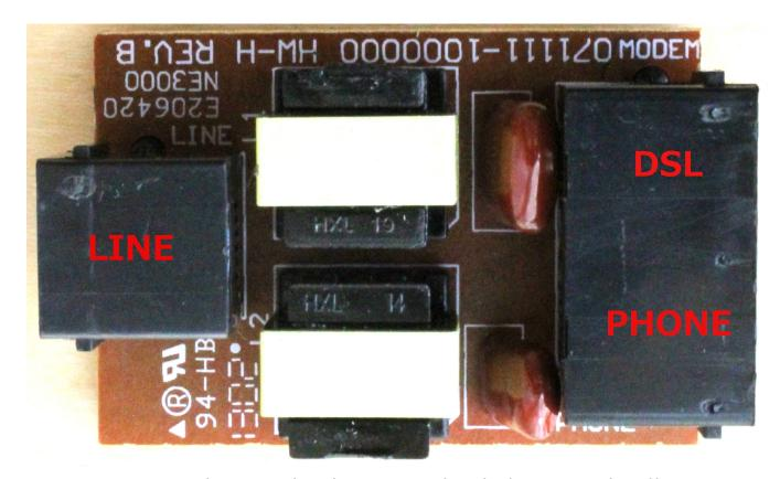
Top View (Line Input (RJ14), DSL Output (RJ45), Phone Output (RJ14))
