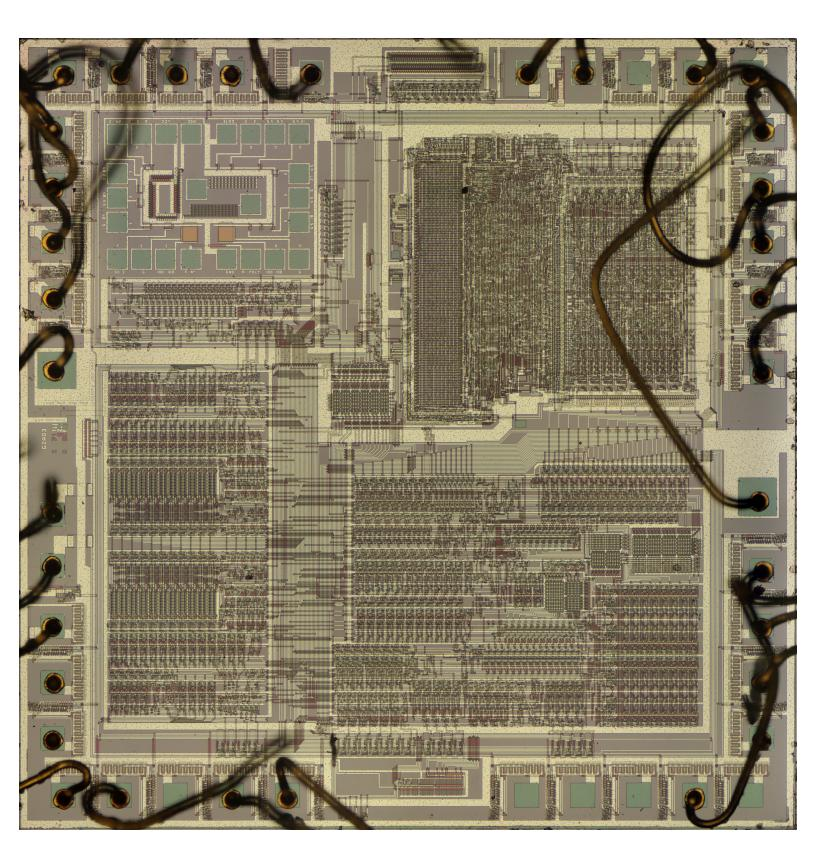
RP2A03 20x Die Photo 16000 x 16288 (261 MP) 6400% (64x) Tolerant Synthesized by Hugin
